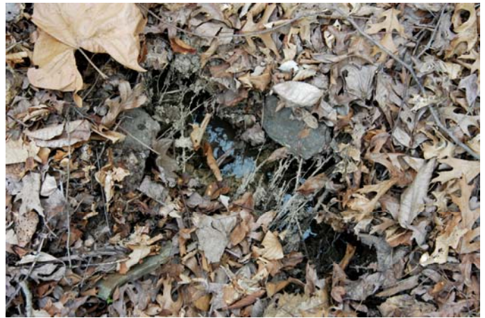
Figure 12. Incipient ground cracking due to minor slippage marginal to main slide. Note water in crack.
